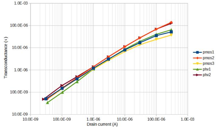
Fig. 3. Transconductance as a function of drain current for each P-channel transistors
