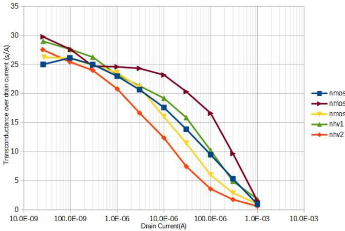
Fig. 6. Transconductance over drain current as a function of drain current for each N-channel transistors
