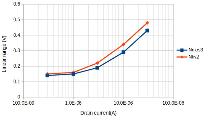
Fig. 7. Linear range as a function of drain current for one low voltage and one high voltage N-channel transistors
