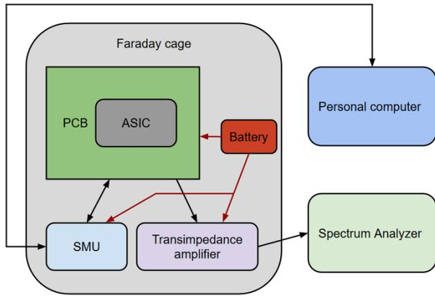
Fig. 2. Setup used for the measurements
