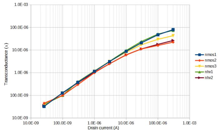
Fig. 5. Transconductance as a function of drain current for each N-channel transistors
