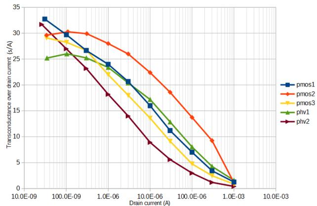
Fig. 4. Transconductance over drain current as a function of drain current for each P-channel transistors
