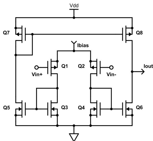
Fig. 1. OTA schematic. Q1 and Q2 are the different DUT, while the rest of the transistors are fixed.
