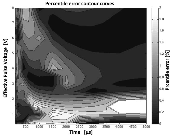
Fig. 10. Simulation error contour plot in the  $T_S \cdot V_{S\_EFF}$  plane.
