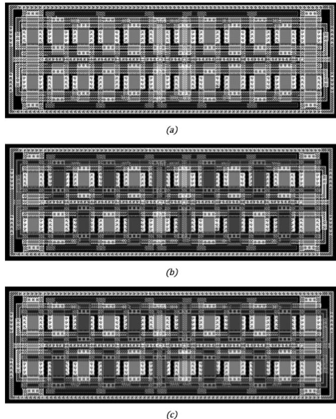
Fig. 5: Layout of the Miller differential Pair. In (b),(c), in dark grey the transistors of each  $M_{1a}$ ,  $M_{1b}$  of Fig. 4.
