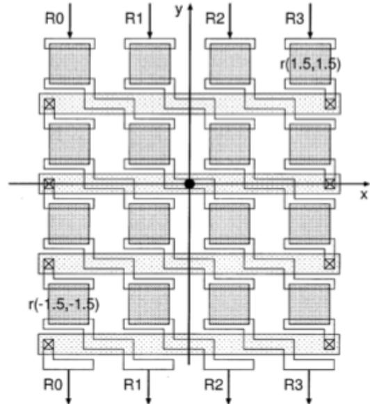
Fig. 6: Layout scheme for the resistors array.
