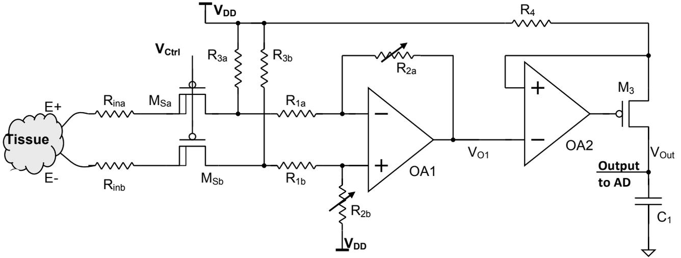
Fig. 3. A scheme of the proposed integrator.  $M_{Sa}$ ,  $M_{Sb}$ ,  $M_3$  bulks are connected to  $V_{DD}$ .
