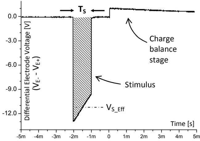
Fig. 2. A measured stimulus pulse. The objective of the proposed circuit is to measure the shaded area.
