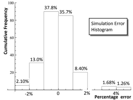
Fig. 9. Simulation error histogram for 250 different pulses, varying also  $R_2$  between its 4 possible values.
