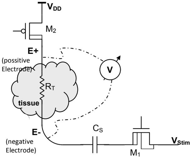
Fig. 1. A simple circuit to deliver a stimulus to cardiac tissue.  $M_1$ ,  $M_2$  are very wide transistors, and  $C_S$  is a series safety capacitor. The voltmeter shows where the pulse amplitude is measured.
