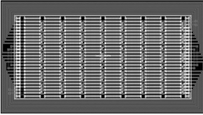
Fig. 7. Layout of the resistor array.
