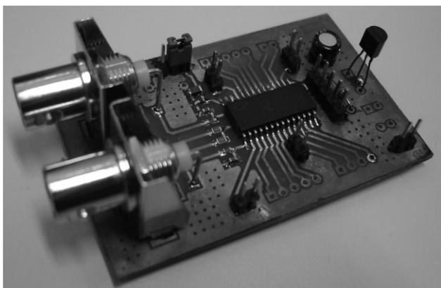
Fig. 4. Custom PCB used to implement the cardiac sense channel.
