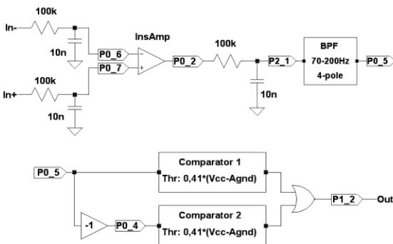
Fig. 2. Simplified schematic of the Cardiac sensing channel implemented in the PSoC, showing on-chip and off-chip signal paths.
