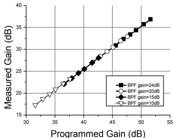
Fig. 6. Linearity Gain test with a CENELEC signal under different BPF and INSAMP programmed gains.
