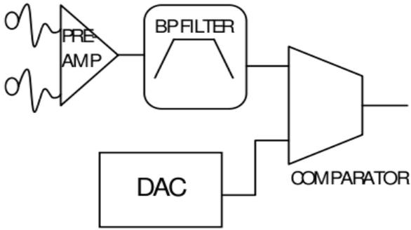
Fig. 1. Block diagram of a typical cardiac sense channel.
