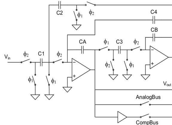
Fig.3. Schematic figure of the filter block implemented in the PSoC, depicting programmable capacitors and clock phases.
