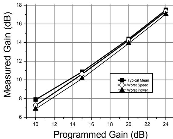
Fig. 10. Measured Gain with the test signal versus Programmed Gain. The upper trace corresponds to the circuit with Typical Mean Transistors. The middle corresponds to the circuit with Worst Speed Transistors. The lower corresponds to the circuit with Worst Power Transistors. Vcc is nominal.
