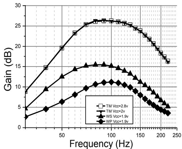
Fig. 9. Frequency response plot of the SC filter. Typical, worst speed and worst power transistors were used, as well as operation under different supply voltages.
