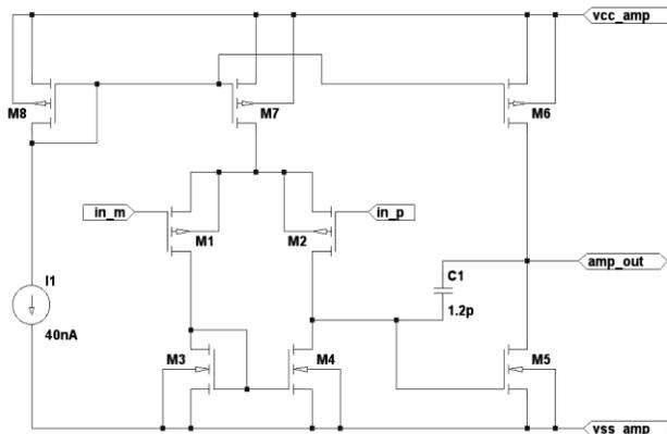
Fig. 8. Schematic of the Miller OpAmp employed in the SC filter.
