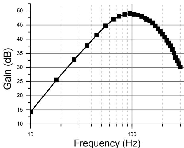
Fig. 5. System frequency response programmed at 54dB gain.
