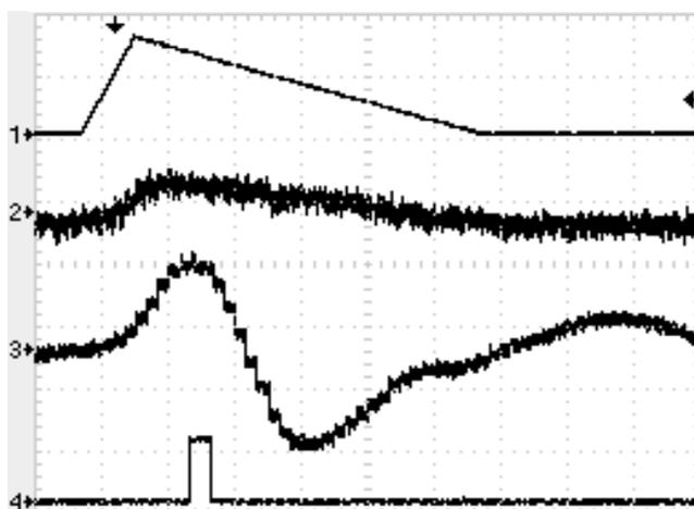
Fig. 7. Oscilloscope capture of the system response to the standard test signal Trace 1, CENELEC signal, in a 200mV/div scale. Trace 2, Insamp out after RC and divisor, 50mV/div. Filter output shown in the middle lower trace (100mV/div), and comparator output in the bottom (5V/div). Time scale is 2.5ms/div.
