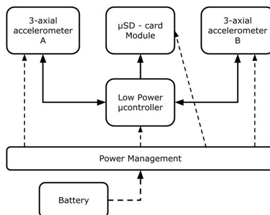
Fig. 1. Block diagram of the physical activity estimation prototype.
