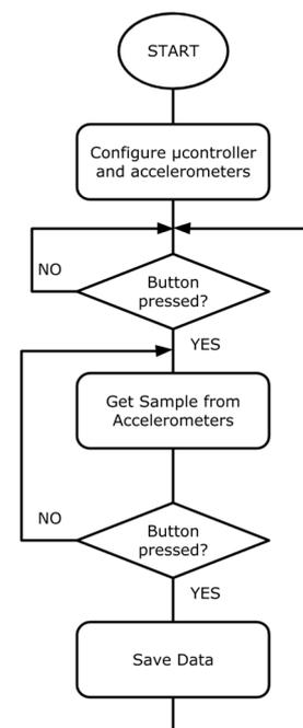
Fig. 4. Simplified diagram of the implemented firmware for data collection.
