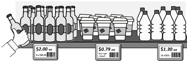
Fig. 1 An Electronic Shelf Label (ESL) is used by retailers for displaying product pricing on shelves substituting printed price tags. The product pricing is remotely updated from a central server.
