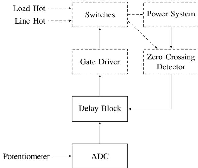
Fig. 3. Top level blocks for the UHV dimmer. *Load Hot* and *Line Hot* are the dimmer terminals that connect to the load and to the grid respectively as shown in Fig. 1. *Potentiometer* is an extra analog input to control the duty cycle. Dashed blocks represent power related blocks and solid blocks represent logic related blocks. Dashed arrows represent UHV connections and solid arrows represent low voltage connections.
