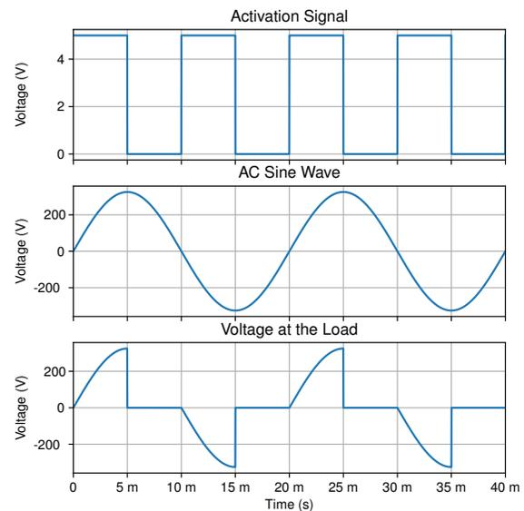
Fig. 2. Load voltage in a phase-cut dimmer.
