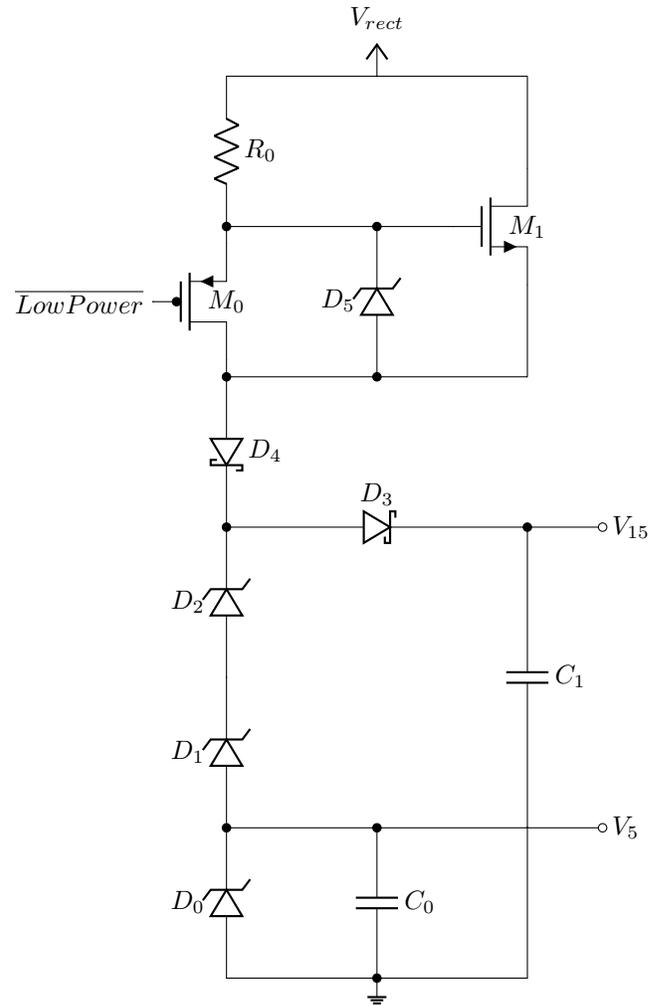
Fig. 6. Power System that delivers 5 V and 15 V from a potentially chopped sine wave voltage.
