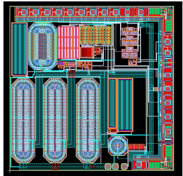
Fig. 12. Top level layout of the UHV dimmer.
